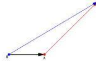
FIG. 19: Evaluation of the potential of a charge moving with constant velocity v in the direction OA . Point O is the retarded position, point A is the current position and B is the observation point. \vec{R}' = \vec{OB} , \vec{R} = \vec{AB} . Note that |\vec{R}'|/c = |\vec{R}' - \vec{R}|/v
